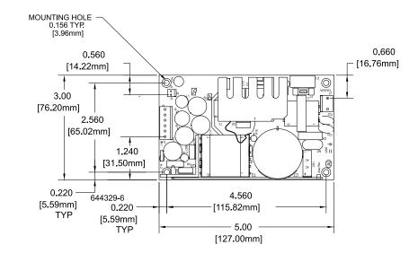
MAX. COMPONENT HEIGHT1.20" [30.28 mm] MAX. LEAD PROTRUSION 0.10" [2.54mm]
